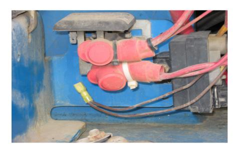
You should hear a distinct audible click sound when you unplug this wire from the separator/isolator. If you do not hear a click, this is another good indication the battery separator/isolator is bad and draining your batteries down.
