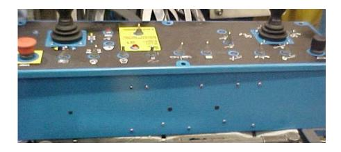
**Step 2:** Check for brake light on ALC board when stroking joystick forward or reverse with foot on footswitch
