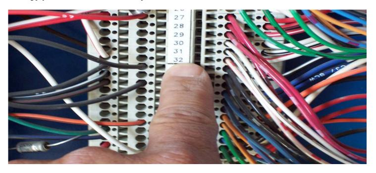
**Step 4:** Check voltage on pin # 23 on engine harness on side of ground control box
