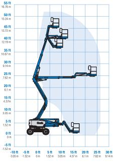
(1) The metric equivalent of working height adds 2m to platform height. The imperial equivalent adds 6ft to platform height. (2) Gradeability applies to driving on slopes and may vary depending on options and machine configurations.
